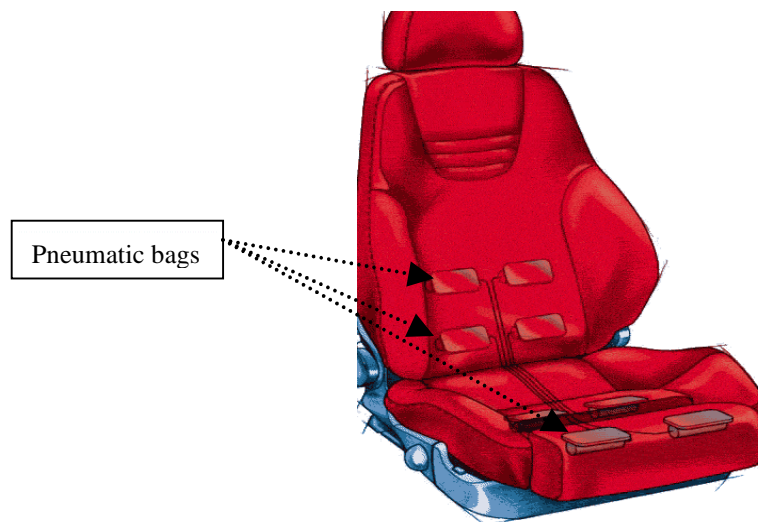
Figure 16: Air pressure relaxation system
